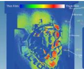
Controlled Lubricant Film Thickness Simulates nozzle quantity and placement, spray pattern volume, angles, and spray film thickness. Control how much lubricant you are applying to each area of the die.
